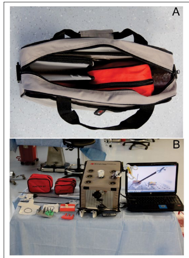
Figure 1. (A) The portable carrying bag containing the collapsed laparoscopic trainer and training materials. (B) The portable laparoscopic trainer deployed and running on a computer (not included in kit).
